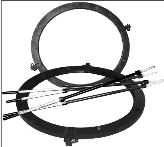
Intended for ensuring convenience and reliability when carrying out technologically safe works on fitting and removing retaining rings from rotors
