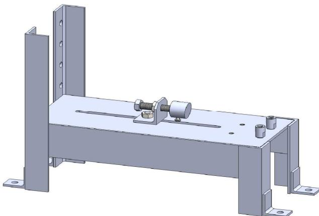
**Bed for wedge machining**
