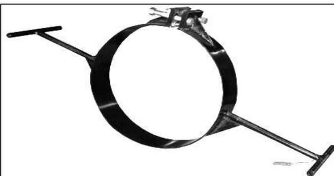
Intended for installing slip rings onto the turbine rotor in the course of repair and renewal works
