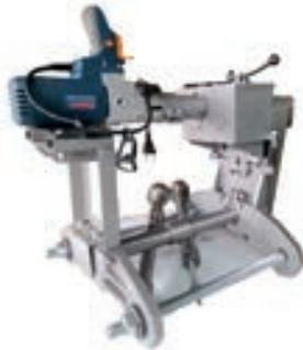
**TURBINE COUPLING HOLE REAMING MACHINE GM.437**
